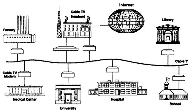
Typical Cable TV High-Speed Data Network
